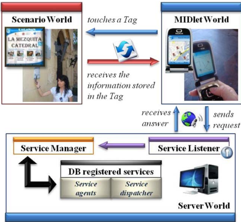
Fig. 2. Architecture for a NFC surfing system
