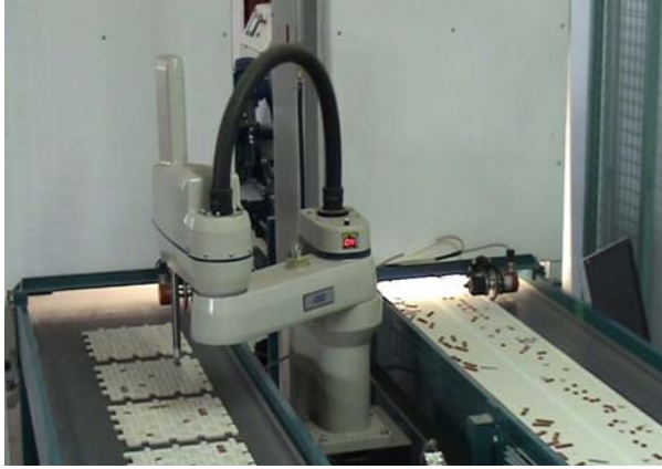
Fig. 2. A photograph of the system. The robot arm picks up tessellae from the right belt and assemble them onto a ceramic tile.
