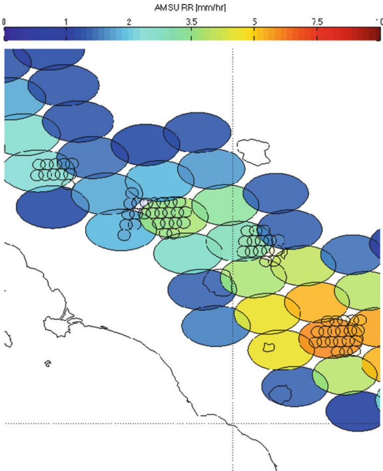
Fig. II.7.25 PC-weighted average on AMSU native grid at 15:30 UTC and on SEVIRI FOVs
