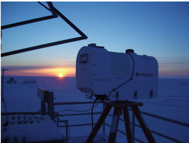
Fig. I.1.4 Picture of the Radiometrics MP-3000A, a multi-channel MWR for temperature and humidity profiling
