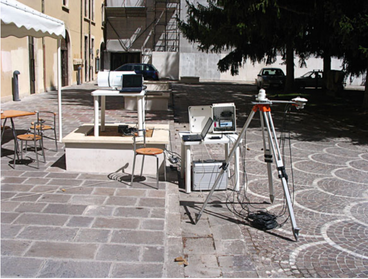
Fig. I.1.3 Picture of the Kipp & Zonen CNR 1 net radiometer ( right ) and the MT5 microwave radiometer ( left ) during the outdoor deployment at ISSAOS 2007 in L'Aquila
