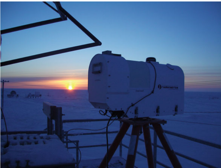
Fig. I.1.4 Picture of the Radiometrics MP-3000A, a multi-channel MWR for temperature and humidity profiling
