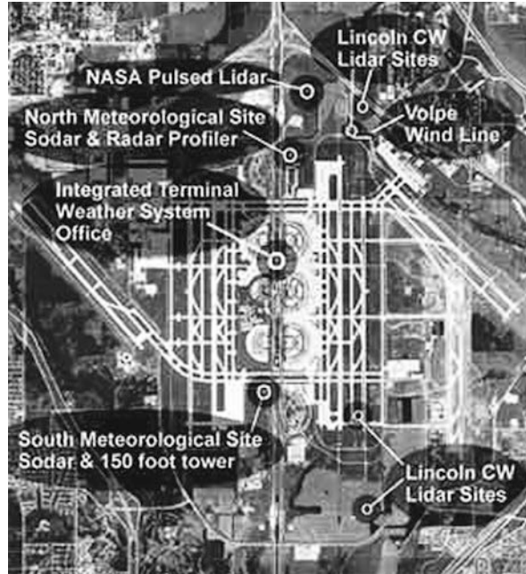
Fig. II.2.8 Instruments deployed during the wake vortex project in Memphis, 1994 (Dasey et al., 1997)
