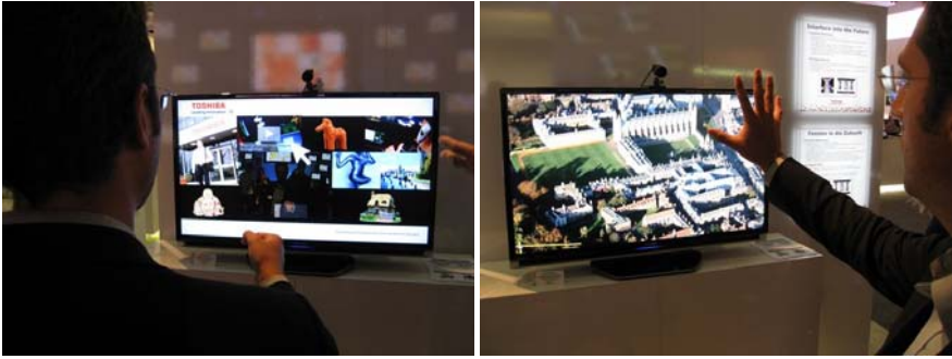
Fig. 9.1 Showcase of the proposed gesture interface. Left: a single camera on top of the display is directed towards the user, who is able to control a screen cursor with his fist. Videos can be selected by hovering over a button. Right: The playback of a video can be stopped with an open hand gesture.
