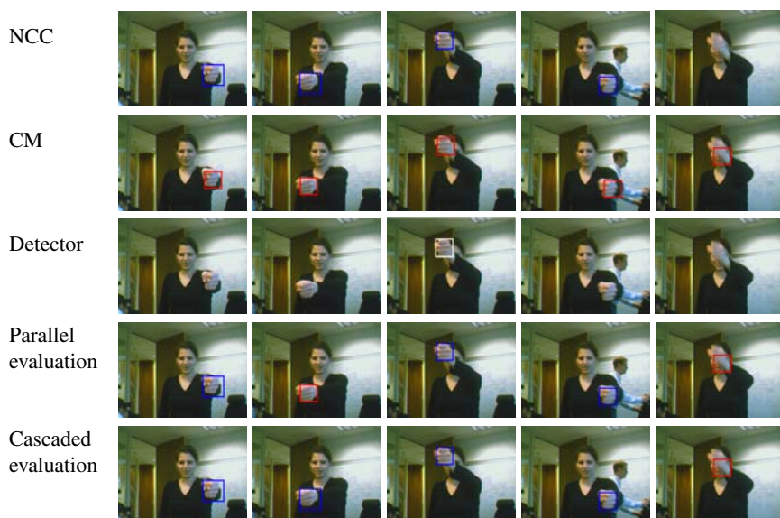
Fig. 9.11 Hand tracking results using NCC and color-motion (CM) observers. Shown are results of individual observers, a detector and parallel and cascaded evaluation. Colors indicate which estimate is used. In this sequence the hand is tracked successfully by both pair-wise schemes with a lower error than with either of the observers.
