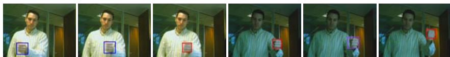
Fig. 9.12 Hand tracking using NCC-CM-M observers in parallel. The NCC observer (blue) is used initially. During motion blur the tracker switches to the CM observer (red). For a couple of frames the M observer (purple) is used, while the light is turned off, before switching back to CM.
