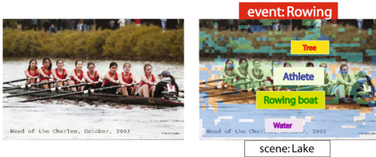
Fig. 6.1 Telling the what, where and who story. Given an event (rowing) image such as the one on the left, our system can automatically interpret what is the event, where does this happen and who (or what kind of objects) are in the image. The result is represented in the figure on the right. A red name tag over the image represents the event category. The scene category label is given in the white tag below the image. A set of name tags are attached to the estimated centers of the objects to indicate their categorical labels. As an example, from the right image, we can tell from the name tags that this is a rowing sport event held on a lake (scene). In this event, there are rowing boat, athletes, water and trees (objects).
