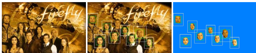
Fig. 3.27 Real time face segmentation using face detection. The first image in the first row shows the original image. The second image shows the face detection results. The third image shows the segmentation obtained using shape priors generated from the detection and localization results.
