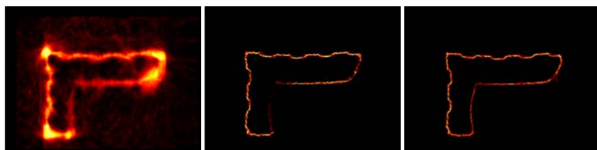
Fig. 11.6 Noise reduction in photo-consistency. Left: a slice of the photo-consistency used in [48] contains falsely photo-consistent regions ( e.g. , near the corners). Middle: occlusion robust photo-consistency proposed in [20] significantly suppresses noise and the correct surface can be accurately localized. One side of the vertical wall is missing due to heavy occlusions. Right: occlusion robust photo-consistency proposed in [8]. The vertical wall is correctly represented.
