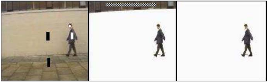
Fig. 3.9 Segmentation in videos using user seeds. The first image shows one frame of the input video with user segmentation seeds (the black and white boxes). The image pixels contained in these boxes are used to learn histograms modelling foreground and background likelihoods. The second image shows the segmentation result obtained using these likelihoods with the method of [7]. The result contains a certain portion of the background wrongly marked as the foreground due to similarity in colour. This error in the segmentation can be removed by the user by specifying a hard constraint. This involves marking a set of pixel positions in the wrongly labelled region as background (shown as the checkered region in the second image). This constraint is used for all the frames of the video sequence. The third image is the final segmentation result.
