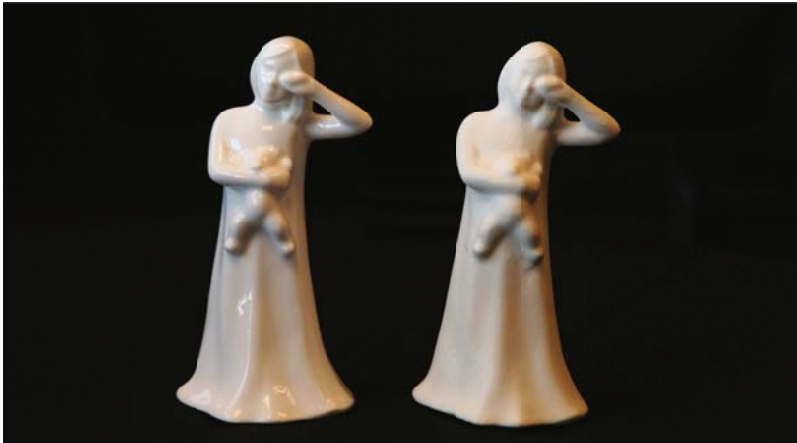
Fig. 11.2 Shading comparison of a porcelain figurine and a manufactured replica obtained using [23]. The original porcelain figurine is shown on the left, while a manufactured replica using the 3D model obtained using [23] is shown on the right. The material of the replica is plaster. See how the replica perfectly imitates the shading component, even though the materials are different.
