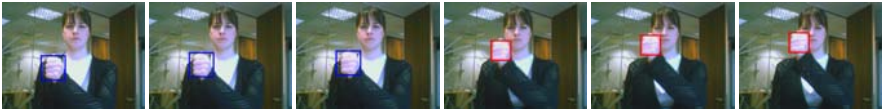
Fig. 9.13 Hand tracking using NCC-CM-FF observers in a cascade. The NCC observer (blue) is used initially, switching to the CM observer (red) during motion blur.
