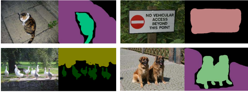
Fig. 7.4 Training Data. A tree is trained on ground-truth labeled images like these above from the MSRC dataset [30], in which each pixel is labelled with an object category (indicated by colors).
