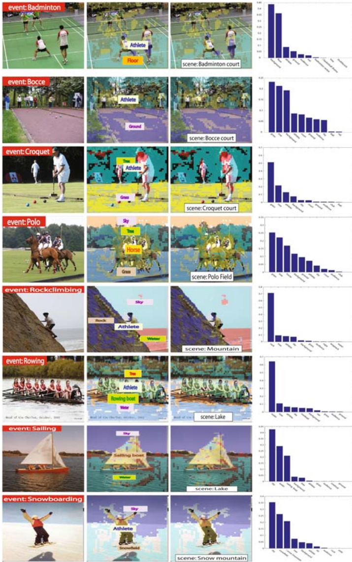
Fig. 6.6 (This figure is best viewed in color and with PDF magnification.) Image interpretation via event, scene, and object recognition. Each row shows results of an event class. Column 1 shows the event class label. Column 2 shows the object classes recognized by the system. Masks with different colors indicate different object classes. The name of each object class appears at the estimated centroid of the object. Column 3 is the scene class label assigned to this image by our system. Finally Column 4 shows the sorted object distribution given the event. Names on the x-axis represents the object class, the order of which varies across the categories. y-axis represents the distribution.
