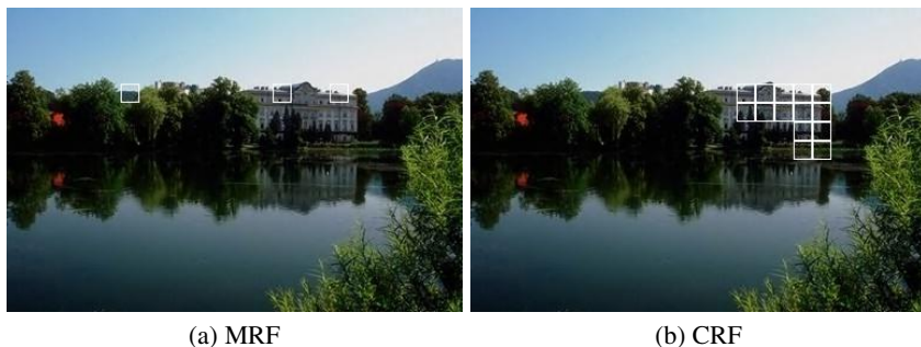
Fig. 4.8 Detection of a building in poor illumination conditions in a test image. CRFs can improve the detection rate while simultaneously reducing the false positive rate.
