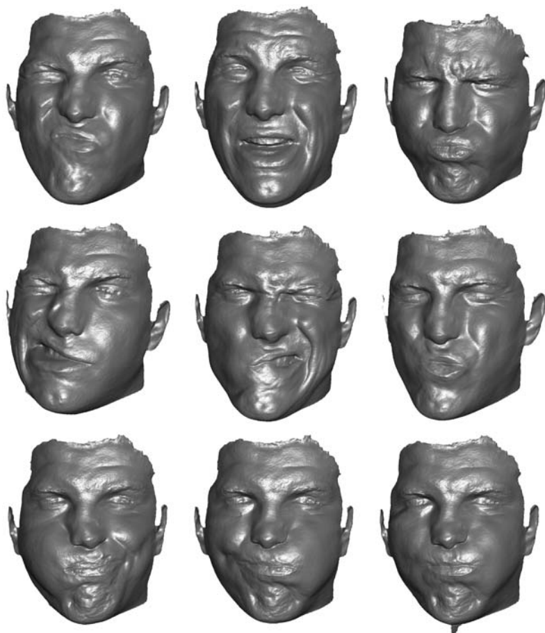
Fig. 12.8 Face sequence. Acquisition of 3D facial expressions using [19] and the shadow processing technique described in this paper. The shadows are processed with the shading regularisation scheme. The full video sequence has more than a 1000 frames reconstructed.
