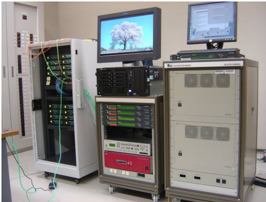
Fig. 8 MPEG-2-based codec system
