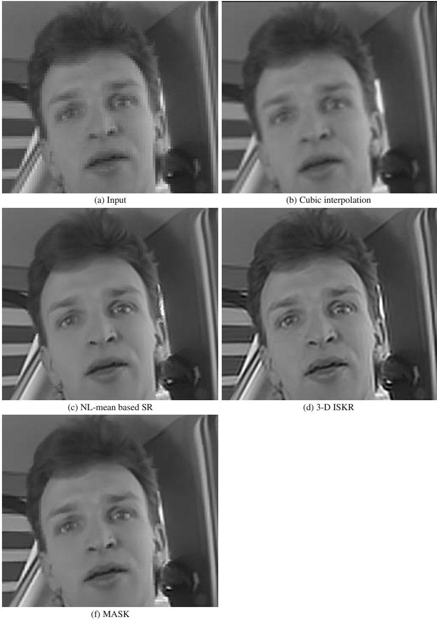
Fig. 11 Spatial upscaling of Car-phone video sequence: (a) input video frames at time t = 25 ( 144 \times 176 , 30 frames) and (b)-(f) the upscaled frames by single frame bicubic interpolation, NL-mean based SR [11], 3-D iterative SKR [13], and MASK, respectively.
