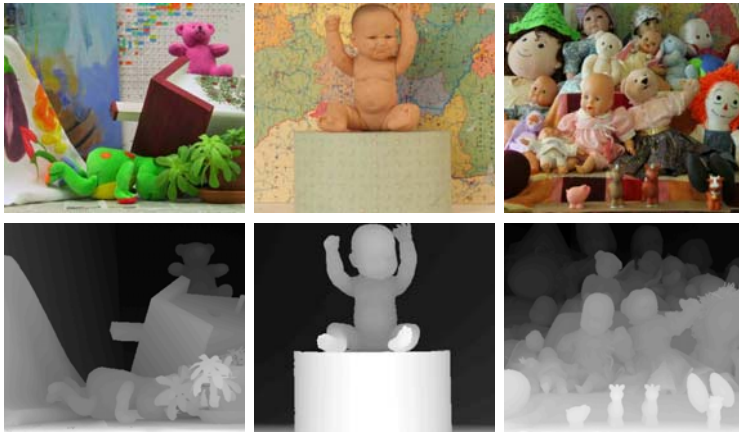
Fig. 4 Left images (Top) of the considered stereo pairs and corresponding ground truth images (Down). From left to right: Teddy, Baby, Dolls.
