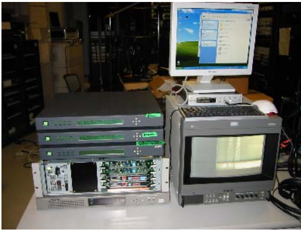
Fig. 19 SHR codec and local monitor for SKF2004
