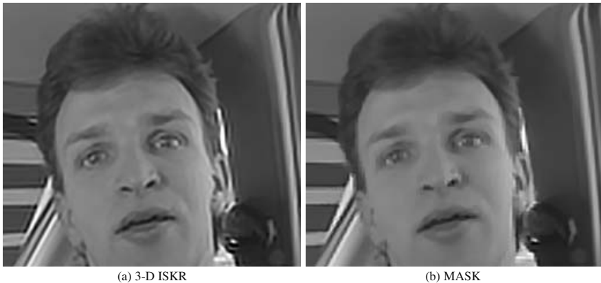
Fig. 12 Spatiotemporal upscaling of Car-phone video sequence: (a) upscaled frames by 3-D iterative SKR [13] at t = 25.5 , and (b) upscaled frames by MASK at t = 25.5 . In this example, we upscale Car phone sequence shown in Fig. 11(a) with the spatial upscaling factor 1 : 3 and the temporal upscaling factor 1 : 2 .
