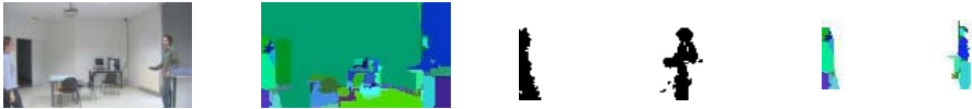
Fig. 7 Object extraction at the top of the pyramid by merging frame segmentation and motion masks. Sequence “Lancé trousse” ©LABRI.
