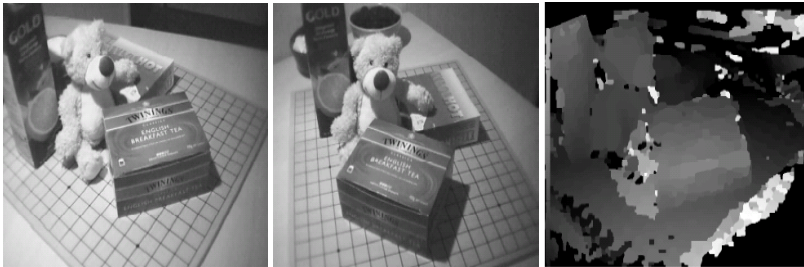
Fig. 11 Test triples and the corresponding depth map, where 1st- and 2nd-column are original images and 3rd-column is the depth map
