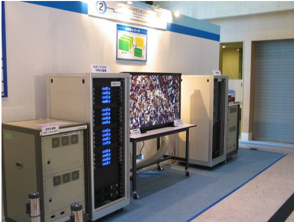
Fig. 10 AVC/H.264-based codec system
