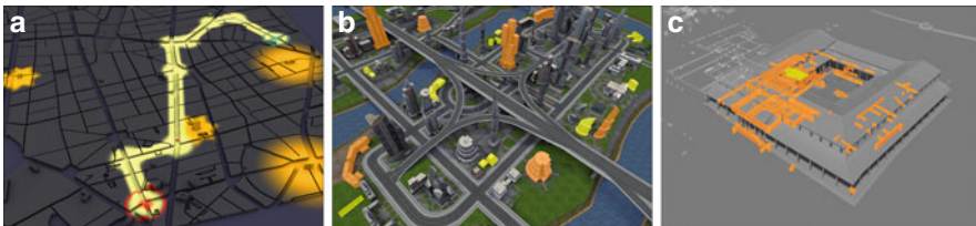
Fig. 6 Application examples of different highlighting techniques applied to 3D GeoVE. (a): Highlighting as navigation aid for routing purposes within a generalized virtual 3D city model of Berlin. (b): Using coloring for building categorization in an artificial virtual city model. (c): Highlighting of finding groups within an interactive digital cultural heritage application
