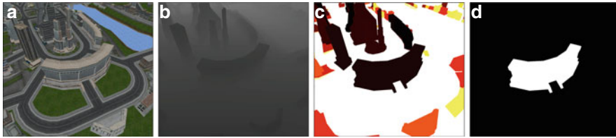
Fig. 4 Image-based representations (scene textures) of the 3D scene that are required by the highlighting pipeline: color (a), depth (b), color coded object IDs (c) and mask (d) values are derived within a single rendering pass
