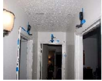
Fig. 4. Height sensors deployed above doorways in a home
