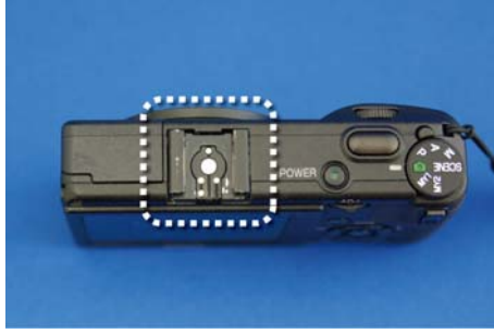
Fig. 3. Hot shoe connector of a high-end compact digital camera (Ricoh GR Digital2). There are 5 signal terminals at center, and ground terminals on each side.
