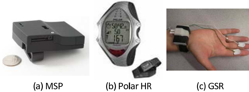
Fig. 1. Sensor Devices included MSP for activity sensing, Polar HR and SHIMMER GSR
