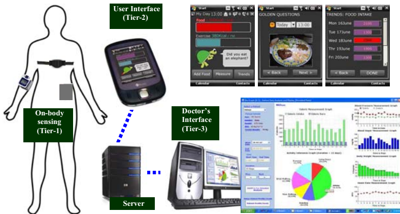
Fig. 1. Jog Falls is a three tier system for diabetes and metabolic syndrome management
