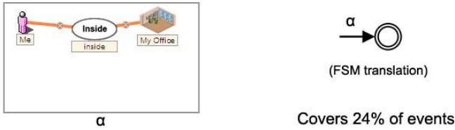
Fig. 4. A Single Scene event: “ I’m in my office ”, translates into a single state FSM that enters the accept state whenever the user is inside his office
