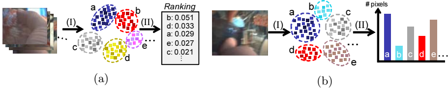
Fig. 3. (a) Clustering pixels of all images of an ADL class and ranking the clusters (features) by their computed information gains, and (b) clustering color pixels of an image and constructing a histogram from the clusters
