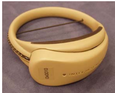
Fig. 1. The Intel iBracelet RFID Reader
