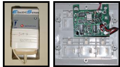
Fig. 2. Left: The signal generating plug-in modules. Right: Inside back cover of the outlet housing the signal generating circuitry.
