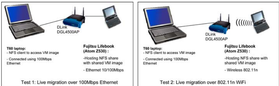
Fig. 3. Two test environments used to capture live migration timings
