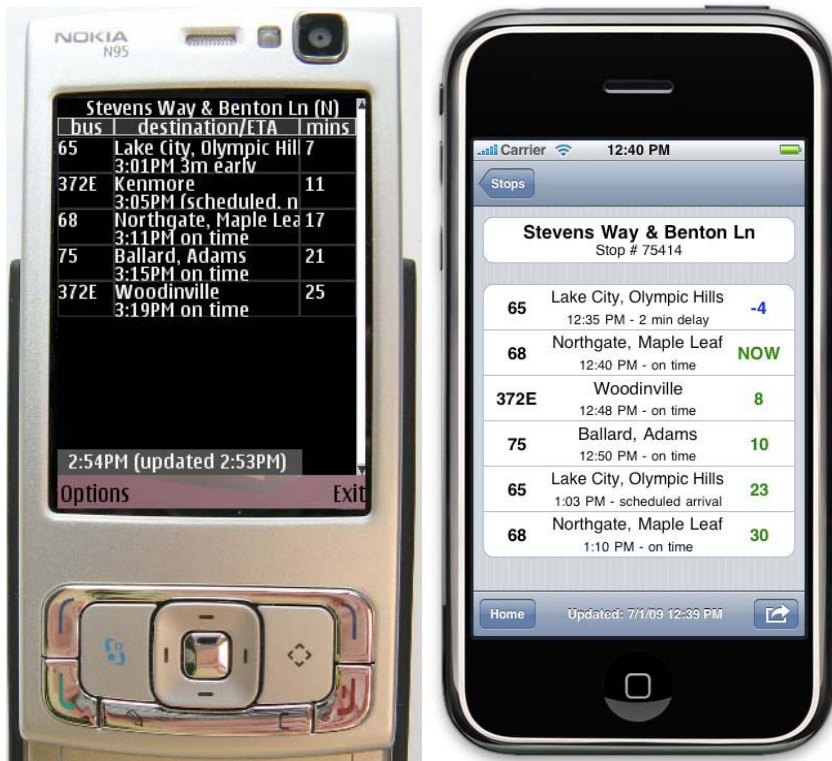
Fig. 1. The current OneBusAway mobile interfaces show real-time arrival information for both Nokia (left) and iPhone (right) platforms, among others
