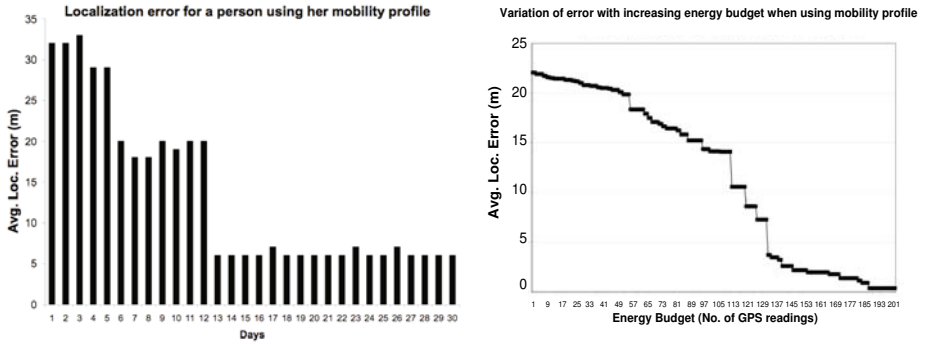
Fig. 8. (a) ALE using individual mobility profile. (b) Variation of ALE with increasing energy budget
