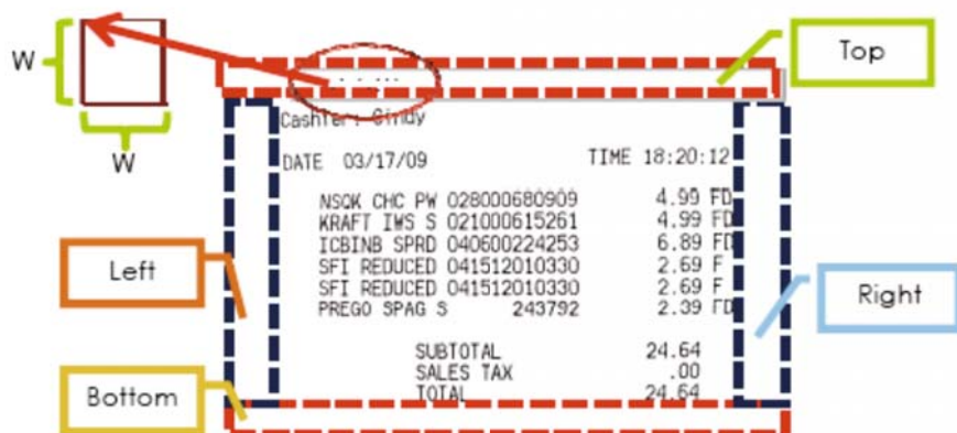
Fig. 4. A perfectly aligned receipt with noise dots located within the top margin and circled by a red ellipse. A W \times W local box is defined to help filter out the noise dots.
