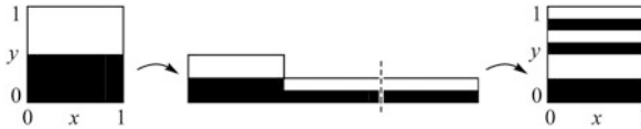
Fig. 2.10 A single iteration of the baker’s apprentice map for N = 1 (the most “skilful” apprentice)
