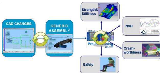
Fig. 2. Integrated solution: from CAD changes to FE models
