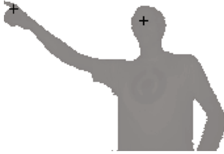
Fig. 3. Segmented image of the user with the detected locations of the head and hand marked by crosses. The time-of-flight camera measures the three-dimensional positions of these points, which are then used to compute the pointing direction.
