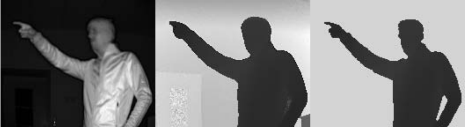
Fig. 2. Sample image taken with a MESA SR4000 TOF camera. The leftmost image shows the intensity data. The range image is given in the center, and the resulting segmentation is shown on the right.
