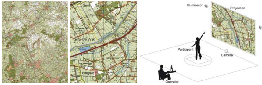
Fig. 3. The whole and a part of the map that the participants had to manipulate and the set-up for this investigation. The operator sat in the back, out of view.
