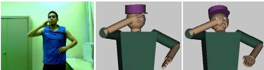
Fig. 8. Augmenting motion capture with gesture models. Left: Input image. Middle: Tracking without gesture model: the hand shape is not captured to meet real-time computation constraints. Right: The gesture model augments the motion capture with fingers movements.
