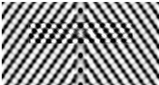
Fig. 2.4 Atomic structure of the 70.5^\circ [110], {112} symmetrical tilt grain boundary in molybdenum. The spacing between parallel rows of atoms is 0.25 nm. The bright belt in the centre of the image is computer-simulated structure [69]. (T. Vystavěl, with permission)
