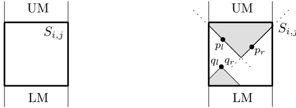
Fig. 1. Definition of regions UM and LM of a square S_{i,j} (left figure). An example of a sandglass (the shaded area) for the case where q_l = q_r . For the upper sandglass, also the lines with slopes 1 and -1 are depicted (right figure).
