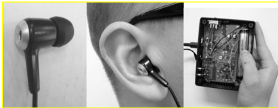
Fig. 1. ARA headset used in the study. Left: In-ear headphones equipped with microphones. Middle: Headset fitted in ear. Right: ARA mixer (Picture taken from [33]).
