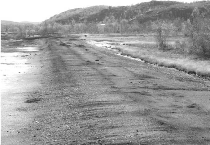
Fig. 2.20 Former roast beds, Sudbury, Canada. Roasting involved piling sulfide ore on beds of wood and igniting it. The forest grows right to the edge of the old roast yard. Metal dispersion from the roast beds has occurred into local soils and plants
