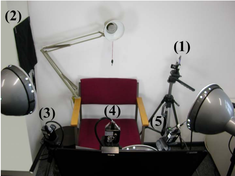
Fig. 1. Experimental setup with larynx camera (1) against black background (2), left (3), center (4) and right (5) camera
