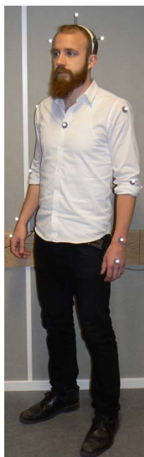
Fig. 4. A Spontal subject rigged with 12 reflective markers
