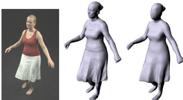
Fig. 8 Input frame (l) and reconstructions using a detailed (m) and a coarse model (r). Although the fine details on the skirt are due to the input laser scan (m), even with a coarse template, our method captures the folds and the overall lifelike motion of the cloth (r)
