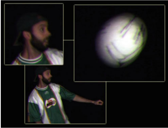
Fig. 5 Using staggered camera triggers and nearest neighbor interpolation produces an interpolated image significantly better than a simple cross-dissolve ( blending )
