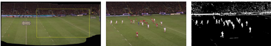
Fig. 7 Difference keying. The camera image ( middle ) is compared against a spherical panorama of the scene ( left ) giving the key ( right )
