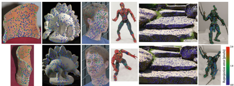
Fig. 9 Matched image features are shown for each data set. The colors represent the associated reprojection errors computed after the last bundle adjustment step. See text for more details
