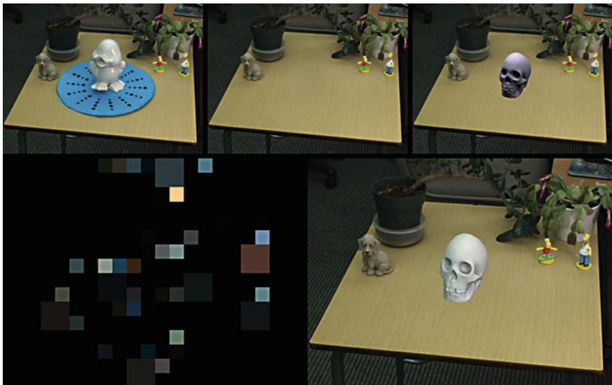
Fig. 8 The top row contains from left to right : the original scene with calibration object, the empty scene and the augmented reality scene with incorrect lighting. The recovered lightmap and augmented reality scene with the correct lighting are shown on the bottom row
