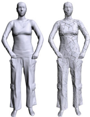
Fig. 3 A surface scan \mathbf{T}_{tri} of an actress (l) and the corresponding tetrahedral mesh \mathbf{T}_{tet} in an exploded view (r)
