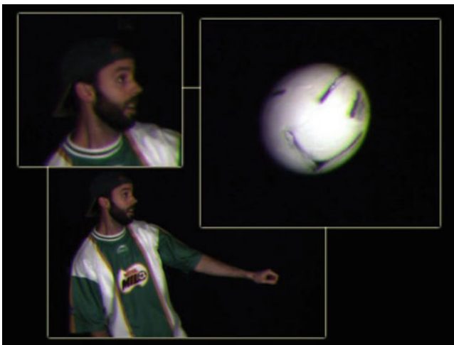
Fig. 6 Using staggered camera triggers and the multibaseline spatiotemporal view interpolation method, we can synthesize a new view without ghosting artifacts
