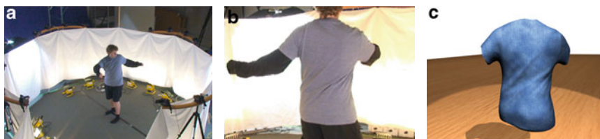
Fig. 1 Garment capture from multi-view video using the method of Bradley et al. [8]. (a, b) Input camera setup with test person. (c) Reconstructed 3-D mesh model of the t-shirt at the same time step. (Images courtesy of Derek Bradley, University of British Columbia, Vancouver)
