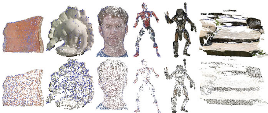
Fig. 5 Top : Patches reconstructed by PMVS at level L of the pyramid. Bottom : Subsets of these patches that have successfully generated feature correspondences after sub-sampling
