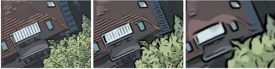
Fig. 7. Level of abstraction by means of trilinear filtering. The viewpoint distance decreases linearly from left to right. The greater the viewpoint distance, the fewer details are depicted at the roof of the building and the tree
