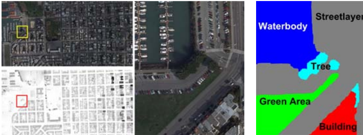
Fig. 1. A pair of images extracted from the dataset San Francisco consisting of color and height information, and the corresponding semantic description of the sub-image (highlighted rectangles).
