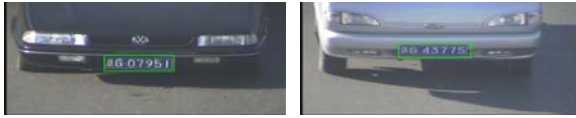
Fig. 3. An illustration of the license plate localization based on the Adaboost classifier
