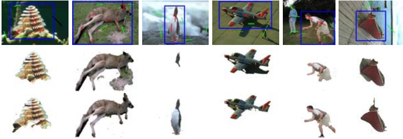
Fig. 3. Segmentation results of GrabCut and proposed iterated graph cuts. The first row shows the original images with seeds. Red and green strokes represent the object and background seeds for graph cuts. User inputs for GrabCut are denoted by blue rectangles. The second row shows the results of GrabCut . The third row shows the results of iterated graph cuts. The proposed method can segment more accurately the desired objects than GrabCut.
