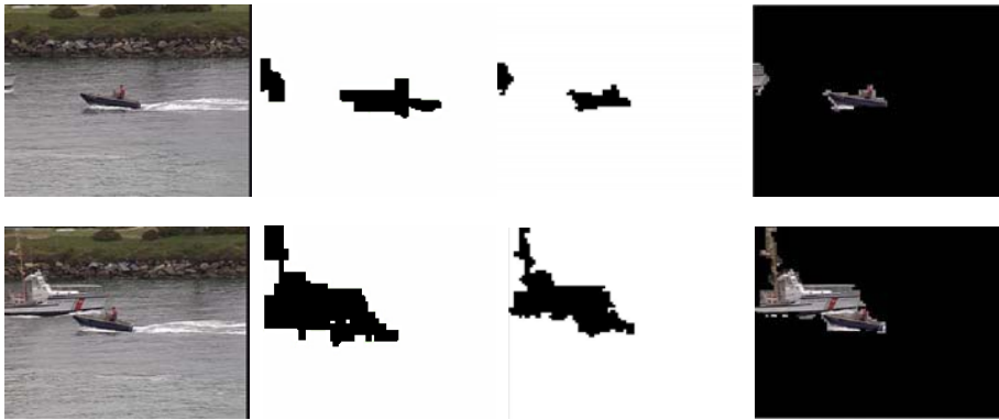
Fig. 5. The result of segmentation in [2]’s approach and the proposed approach. The first row is the 1st frame in Coastguard and encoded as I-frame. The second row is the 37st frame and encoded as P-Frame.
