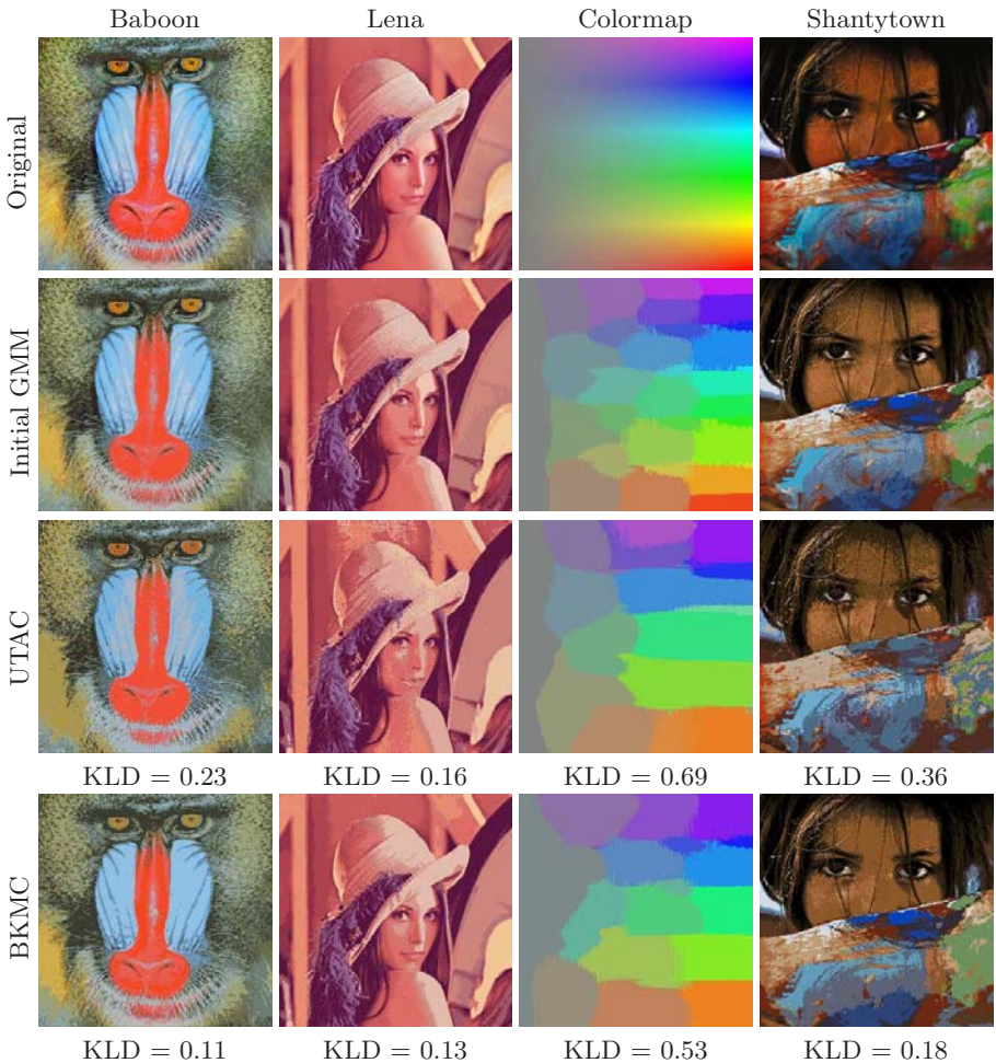
Fig. 3. Application of GMM simplifying algorithms (UTAC and BKMC) to clustering-based image segmentation. The BKMC algorithm provides the best results (visually and according to the KLD value).
