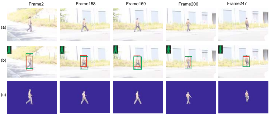
Fig. 3. Tracking and segmentation results for the outdoor sequence. (a) Input images. (b) Initial bounding boxes (in red) generated by the tracker, optimal bounding boxes (in green) and gait models (phase) calculated by the optimal path searching using shape sequence matching. (c) Segmentation results by embedding the shape priors in the Min-Cut algorithm.
