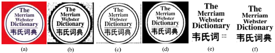
Fig. 13. (a) Original image (b) Niblack's Method (c) Sauvola's Method (d) Chang's Method (e) Kasar's Method (f) Proposed Method
