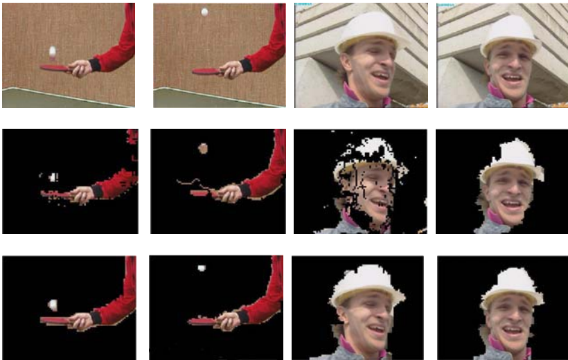
Fig. 7. The results of moving object segmentation for tennis and foreman sequence. The first row is origin picture, the second is intermediate result, the last is final result. The first and second column is 12 st and 17 st frame in tennis sequence respectively. The third and fourth column is 12 st and 17 st in foreman sequence respectively.
