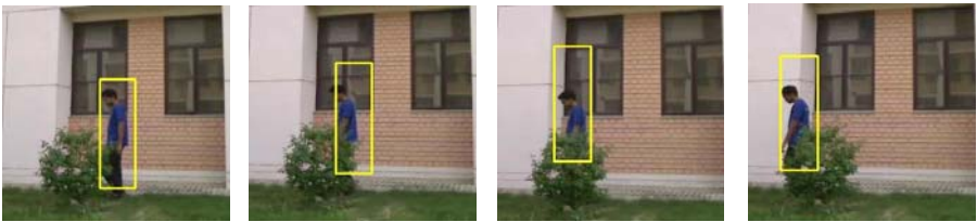
Fig. 2. The sequence of images demonstrates the divergence of mean shift tracker from the target in presence of scene occlusion
