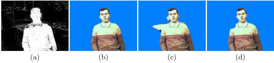
Fig. 3. Segmentation results. (a) the combined probability map of global and per-pixel color models; (b) foreground obtained with both confidence and adaptive thresholds; (c) foreground obtained without using confidence ( \hat{\omega} \equiv 1, \check{\omega} \equiv 0.5 ); (d) foreground obtained without using adaptive thresholds ( T_i^F = T_i^B = T_i ).
