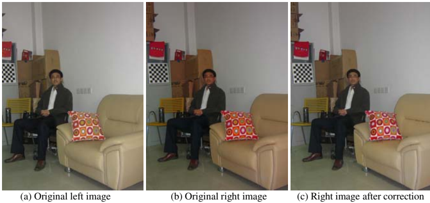
Fig. 6. (a) and (b) are the original image pair taken from stereo cameras. (c) is the right image after color correction.
