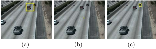
Fig. 2. Result of the original mean shift tracker (a), original mean shift tracker using the 10% scale adaptation (b), and the proposed method (c)
