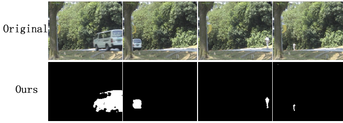
Fig. 4. Detection results from the Campus sequence, which contains large-area waving leaves. The first row contains the original video frames. The second row contains the detection results obtained by our method.
