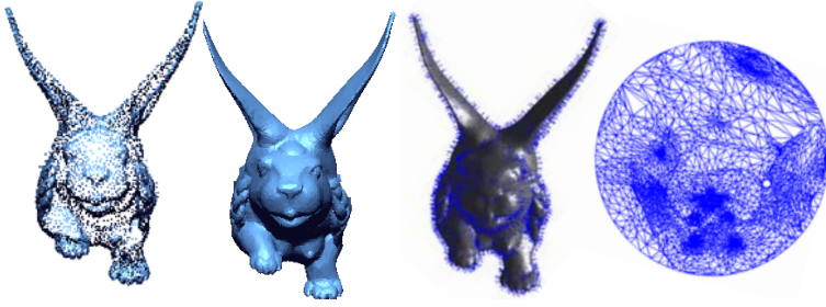
Fig. 1. a|b|c|d. (a) A partial point-clouds 3D model. (b) Shaded 3D model. (c) Normals on the 3D model. (d) 2D mesh parameterization with fixed boundary of this 3D model.
