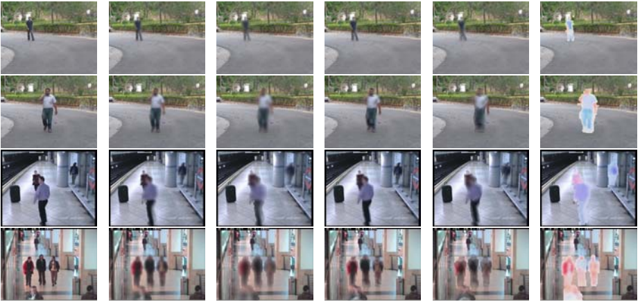
Fig. 4. The first column shows the clear frame. The next five columns show the output of Blur-2, Blur-4, LIC-10, LIC-20, and Blur-2 followed by an intensity space compression, in that order
