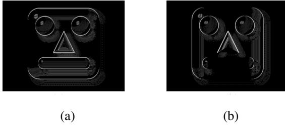
Fig. 5. The reflectance derivatives are larger than the shading derivatives in our weighted map. (a) W_x image. (b) W_y image.
