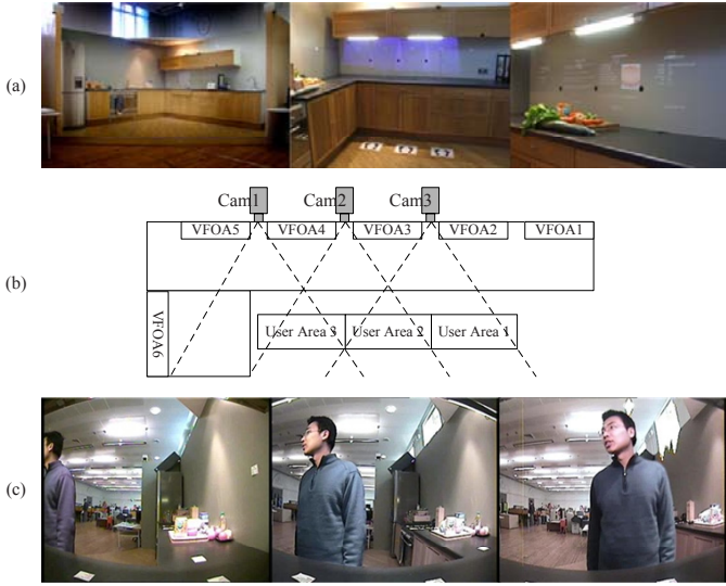
Fig. 1. (a) The Ambient Kitchen, the four displays on the walls, and the markers; (b) the layout of the VFOAs, cameras and areas; (c) the images captured by 3 cameras when the user is standing in area 2
