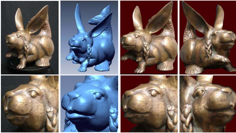
Fig. 5. \frac{a|b|c|d}{e|f|g|h} High-fidelity 2D/3D texture registration results using the suggested method. (a)(e) Camera photo for the real 3D object. (b)(f) The scanned 3D model. (c)(g) and (d)(h) Final results of multiple image registration on the 3D model.
