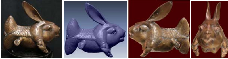
Fig. 6. a|b|c|d High-fidelity 2D/3D texture registration results using the suggested method. (a) Photograph. (b) The scanned 3D model. (c)(d) Final results of multiple image registration using the suggested method. Look from different viewpoints.
