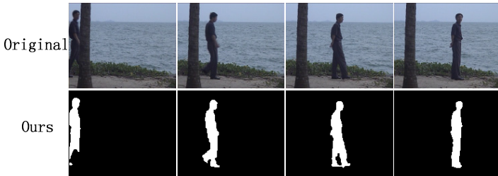
Fig. 3. Detection results from the Water_Surface sequence, which contains the ocean waves. The first row contains the original video frames. The second row contains the detection results obtained by our method.
