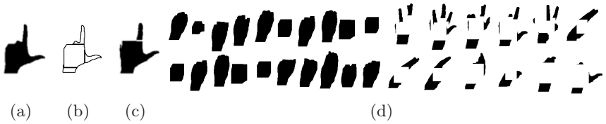
Fig. 3. A hand silhouette (a) is broken into parts, indicated by their outlines in (b). The reconstruction of this silhouette using the dictionary of parts in (d) is shown in (c). This dictionary was learned from the training set described in Sect. 5. Each part is displayed using the corresponding binary mask, with multiple non-overlapping non-palm parts drawn in the same image to conserve space. We successfully learn semantically meaningful palms and groups of fingers in an unsupervised fashion.
