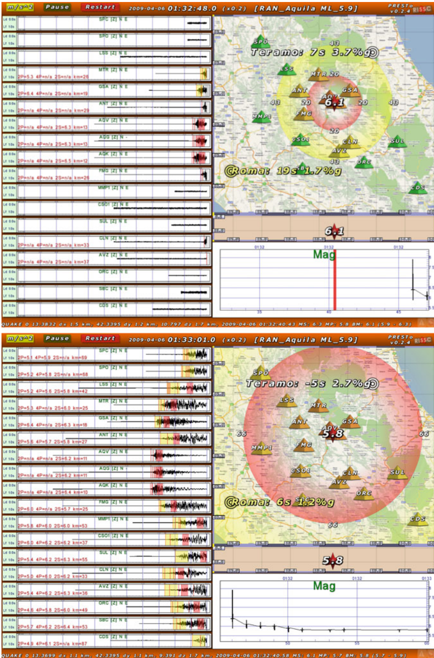
Fig. 7.4 Screen shots of PRESTo during the simulation of the 2009, ML 5.9, L'Aquila earthquake. Top the first estimates of the earthquake source parameters that are affected by a low uncertainty are provided about 7s after the origin time. Bottom the earthquake has been processed for some seconds and the estimates have converged to the final values. This screen shot shows the complete picture of inputs and outputs
