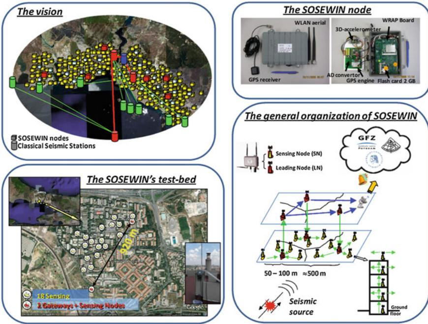
Fig. 6.2 Overview of the self-organizing seismic early warning information network (SOSEWIN)
