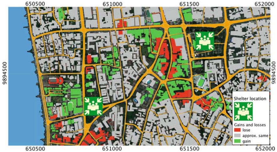
Fig. 11.7 Gains and losses in terms of evacuation time: evacuees departing from green buildings gain more than 10 min because of the shelters; evacuees departing from red buildings lose more than 10 min
