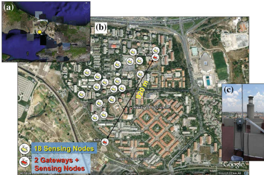
Fig. 14.2 a Location map of Istanbul showing the Ataköy district, where the test-bed SOSEWIN is situated. b The location of the sensing nodes and gateways for the test SOSEWIN in the Ataköy district, Istanbul. c A typical SOSEWIN sensing node installation (from, Fleming et al. 2009)
