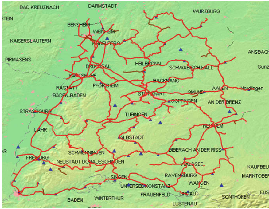
Fig. 8.10 Map of closed ( red ) and speed-reduced ( brown ) railway lines in test area for the simulated earthquake
