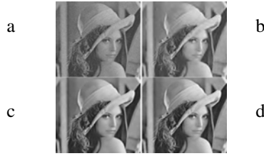
Fig. 2. a) Noisy image, b) filtered images using the decimated wavelet transform, c) the undecimated wavelet transform, d) curvelet transform
