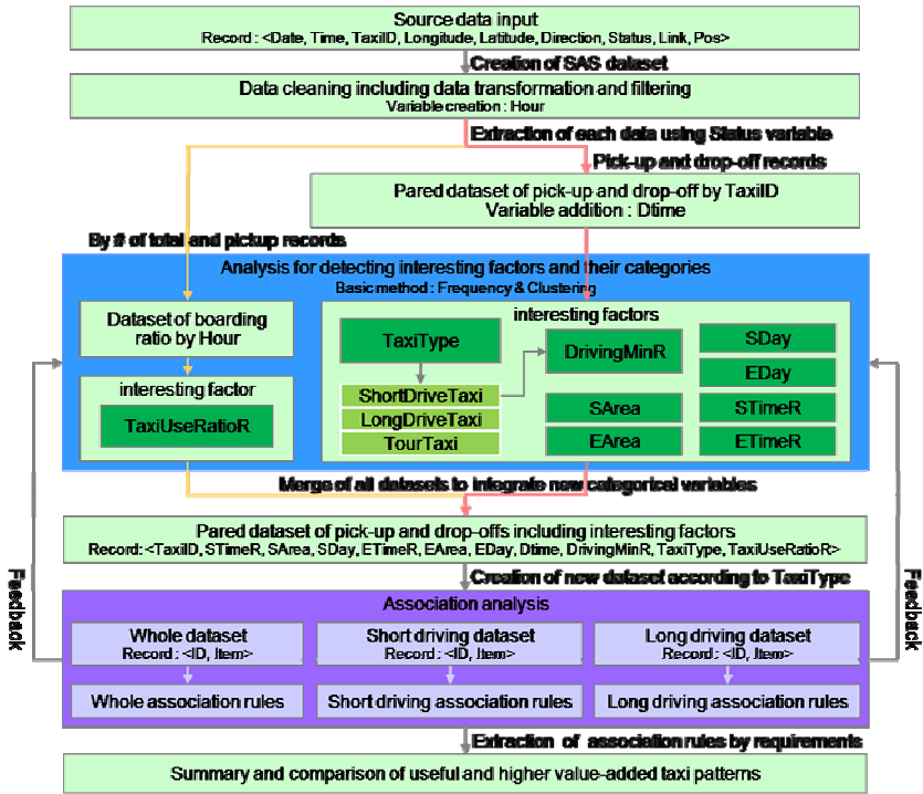
Fig. 2. The analysis processing framework for the association rule mining of taxi records
