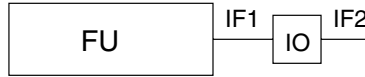
Fig. 1. An IO hardware block translates the interface of the functional unit (IF1) to the desired interface (IF2)
