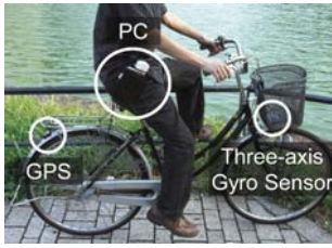
Fig. 1. Bike with GPS, three-axis sensors, and a PC for uploading data
