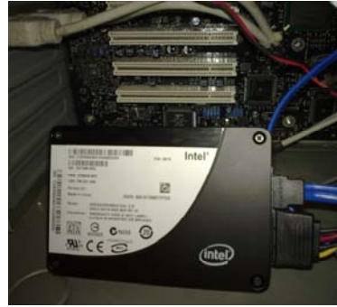
Fig. 2. Connecting SSD to motherboard
