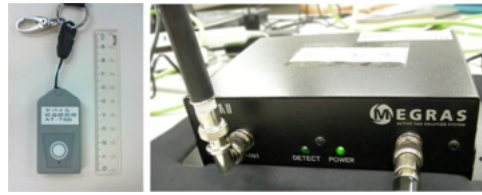
Fig. 1 RFID System (transmitter and receiver)
