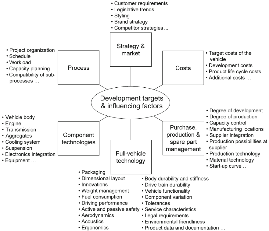
Fig. 1.12 Development targets and influencing factors of automotive full-vehicle engineering processes [15]
