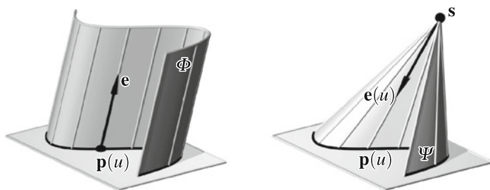
Fig. 3.86 Cylinders and cones are particular types of ruled surfaces. Left a cylinder \Phi is defined by its directing curve \mathbf{p}(u) and the constant direction vector \mathbf{e} of its parallel straight line generators. Right the straight line generators of a cone go through a vertex \mathbf{s}
