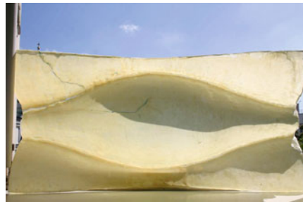
Fig. 7.10 Prototype model of facade element, fibre composite material [62]
