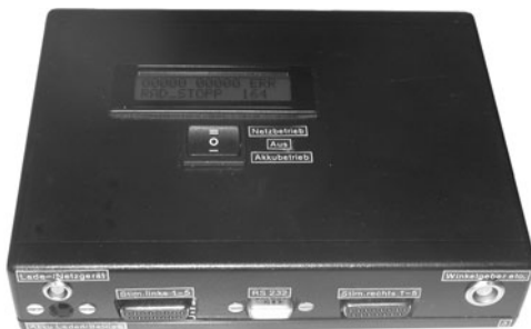
Fig. 11.14 Current controlled 10-channel stimulator for FES cycling and rowing applications
