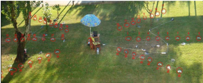
Fig. 3. Nodes distribution according the circular topology, at an outdoor environment
