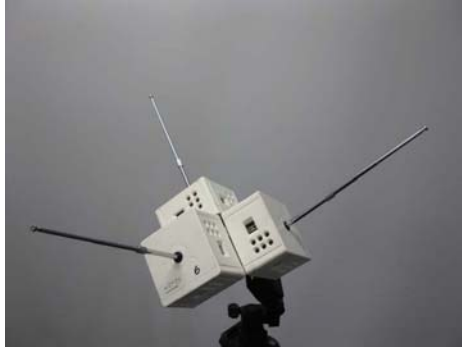
Fig. 1. Antenna array implementation using three XSM nodes
