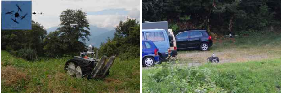
Fig. 1. A Jacobs land robot and an aerial robot cooperating in one of the scenarios at the European Land Robot Trials 2007 (ELROB) in Monte Ceneri, Switzerland. The aerial robot has to find and locate hazard spots like seats of fire, which the land robot then has to reach.
