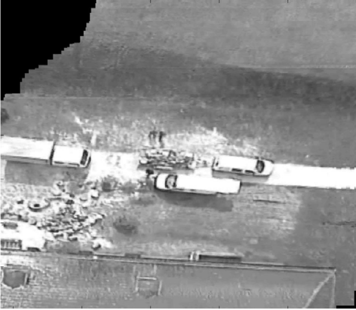
Fig. 2. An image map generated with iFMI in real-time from about 300 images acquired with an UAV. The scene involves several challenges, especially large featureless areas.
