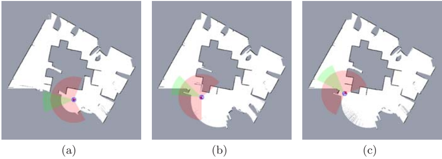
Fig. 8. Successful loop closing using a Hyper Particle Filter (HPF) with 30 particles. (a) Situation right before the loop closing. (b) The robot scans areas that it has visited before; first errors in the map are visible. (c) The HPF closes the loop by switching to a consistent map.
