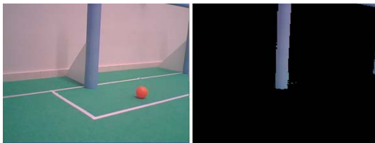
Fig. 1. Colour filtering for the blue goal
