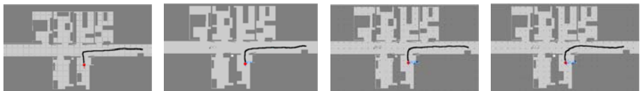
(a) B21 with DWA (b) B21 with A^* ( v_{\max} = 0.45 cm/s) (c) B21 with A^* ( v_{\max} = 0.95 cm/s) (d) Caesar with A^* ( v_{\max} = 3 m/s)
