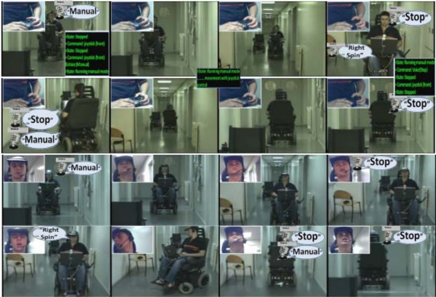
Fig. 8. Real wheelchair movement in a corridor with obstacles using joystick and voice control and using head and voice control
