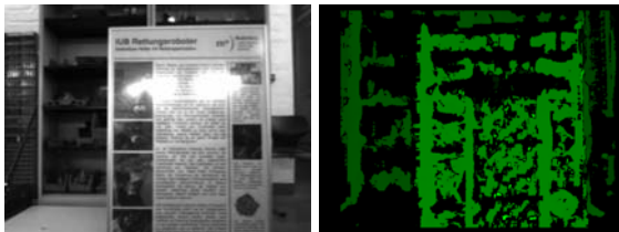
Fig. 3. The left camera image, and the corresponding disparity image of a flat surface with visual features
