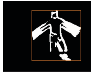
Fig. 14.13. The video mapper input takes essentially the rectangle around the visible pixels.
