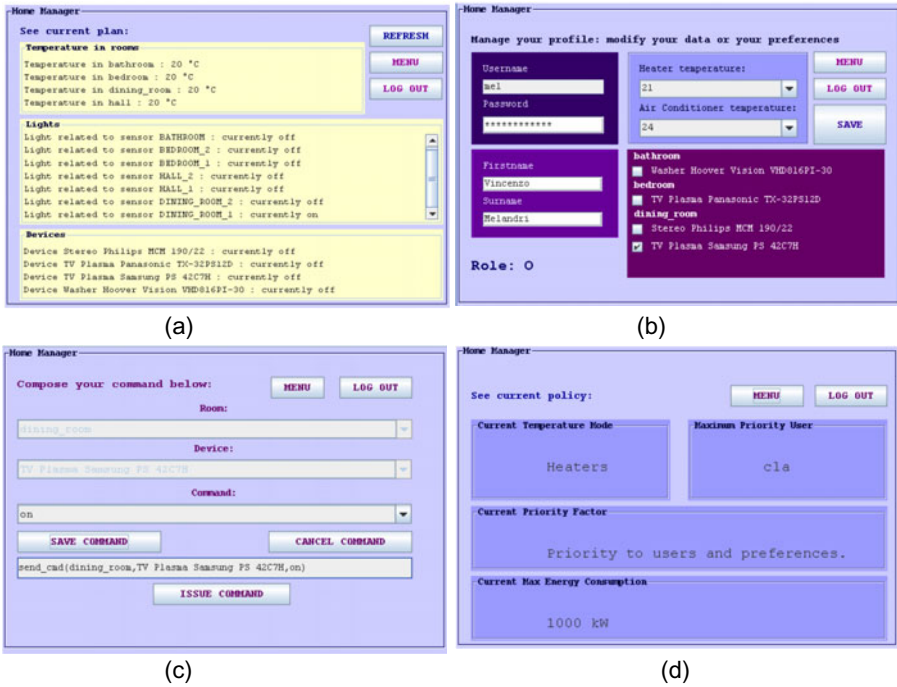
Fig. 7. Some screenshots of HomeManager: a) policy-management interface, b) profile-management interface, c) command interface and d) current-policy interface
