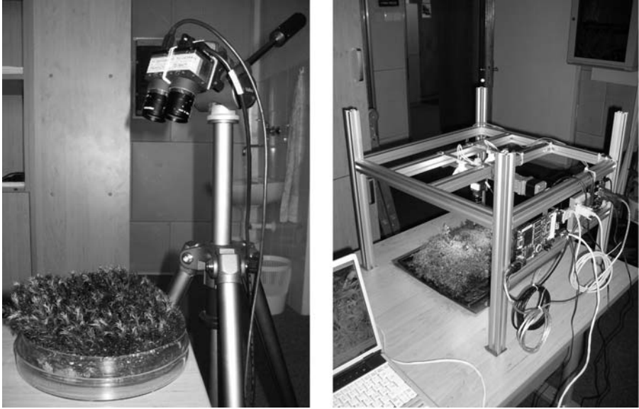
Fig. 2. The pair of cameras mounted on the tripod for mobile use (left) and camera mounted on linear motion with embedded computer for laboratory use (right)
