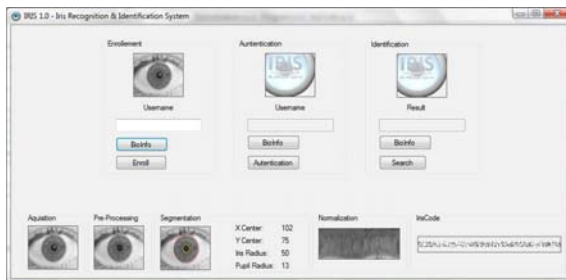
Fig. 11. C# prototype for iris recognition, with enrollment, authentication, and identification functionalities. On the bottom-left corner we see the results of the pre-processing algorithms and the segmentation stage. The bottom-right corner shows the normalization stage results and the IrisCode.
