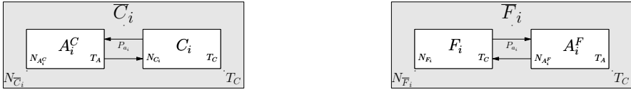
Fig. 1.21 Left: coherence state \bar{C}_i expanded to show sub-states A_i^C and C_i . Right: forward state \bar{F}_i expanded to show sub-states A_i^F and F_i . The average number of robots in each state is shown as N ; T_A is the number of time steps spent in the avoidance states A_i^C and A_i^F .
