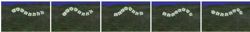
Fig. 2.33 Caterpillar Movement: Several robots are docked in a row and by only moving the hinges of each robot like a caterpillar the organism moves forward.
